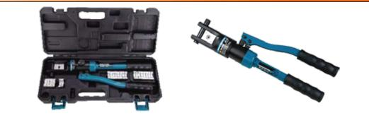
Hydraulic crimping tool is a professional tool for crimping copper and aluminum lugs with different types, a wide range of crimping dies from 4 mm<sup>2</sup> to 1000 mm<sup>2</sup> to suit for different size demand. The main crimping shape is hexagonal, special shape design is provided.
